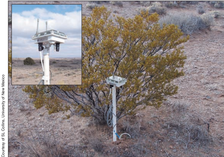
Figure 3. Ecologists are beginning to take advantage of emerging technologies for the remote collection of environmental information. Here one of a network of Sensor Web pods, developed at NASA/JPL, is shown monitoring the microclimate beneath a creosote bush at the Sevilleta Long Term Ecological Research site. Each Sensor Web pod contains six environmental sensors (light, air temperature, humidity, soil temperature and soil moisture at two depths) and wirelessly communicates sensor data to other pods in its local neighborhood, thus distributing information throughout the instrument as a whole. Information is then relayed via a "mother pod" to a laptop and then posted directly on the Internet ( http://sev.lternet.edu/research/SWEETS/index.html ).
